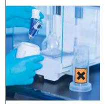
Direct dosing into the target container avoids the spillages which may occur during the manual weighing-in and transfer of the powder. The reduced cleaning effort required further minimizes operator exposure to toxic materials.
