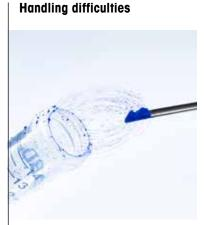
Powders can be hygroscopic, temperature-sensitive, or susceptible to electrostatic charge. External influences make powders tricky to handle, affect the speed of the weighing and the quality and reproducibility of results.
