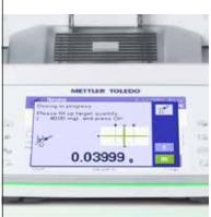
Quantos can dose from 1 milligram to 5 grams of freeflowing powder directly into your target container. The highly accurate dosing process eliminates variability and out-of-specification results.
