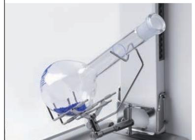
One step dosing directly into the tare container eliminates transfer errors and saves money by minimizing sample loss. Even unusual shaped containers are held securely in place. In combination with the MinWeigh Door™ accessory, ErgoClips help you achieve the lowest possible minimum weight.
