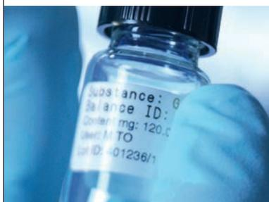
Avoid transcription errors with printouts that conform to all GxP quality standards and provide full traceability. Sample labels with barcodes can also be printed directly from your balance. A Bluetooth® printer placed outside sensitive areas prevents contamination of the printer and the printouts.
