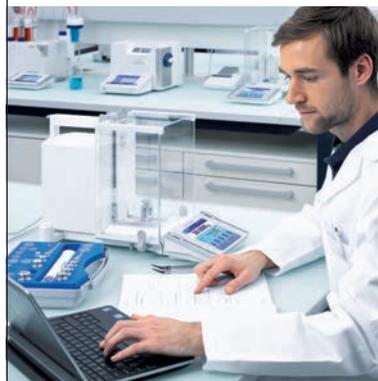
Balance calibration is at the core of accurate weighing results. Each calibration certificate declares the balance's minimum weight and measurement uncertainty – essential information for reliable weighing processes.
