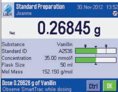
LabX provides step-by-step user guidance on the balance touchscreen so you can be sure your SOP is followed precisely. Centralized instrument management means all your balances automatically display the same SOP instructions to guarantee consistency in your lab.
