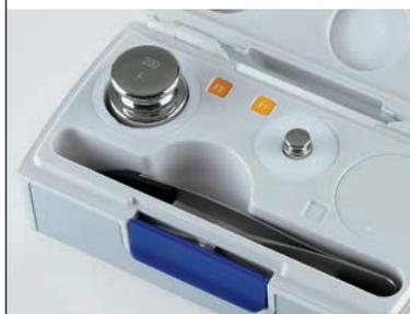
CarePacs® contain just what you need to test your balances in accordance with USP 41 – two test weights corresponding to 5% and 100% of the capacity of your balance. Tweezers, gloves and other accessories are included for professional weight handling.
