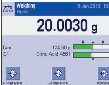
The color-guided SmartTrac™ function makes it easy to dose to your target weight and stay within tolerances. Using the appropriate ErgoClip enables you to dose directly into your container in one easy step.
