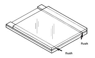
**Note**: The easiest way to check for proper alignment is to run a fingernail across the contact area between the glass plates and spacer. If your fingernail catches or drops as you move from plate to spacer to plate, you must realign the sandwich before proceeding to step 10.
