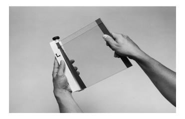
4. Place the right clamp on the right side of the plates, and tighten the clamp screw.
