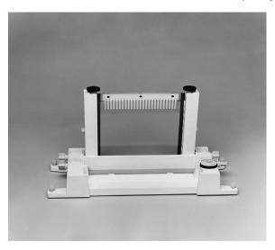
Generally, an overlay solution is not necessary for polymerization when a comb is in place.
