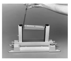
9. Add APS and TEMED to the degassed monomer solution, and pour the solution down the spacer nearest the upturned side of the comb. Pour until all the teeth have been covered by solution. Then properly align the comb in the sandwich, and add monomer to fill completely.
