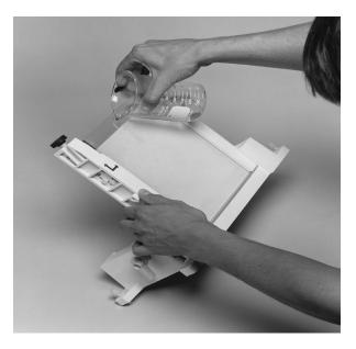
**Note**: If an incubator is not available, molten (75 to 85 °C) agarose can be poured into a room temperature sandwich assembly. This temperature is high enough to prevent premature gelling of the agarose, yet low enough to prevent cracking of the glass plates.
