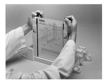
8. Loosen one clamp screw slightly. While pushing down on the spacer with one finger, tighten the clamp screw finger-tight with the other hand (see photo). This will insure proper sealing when solution is poured. Tighten the other clamp screw in the same manner. It is important to visually inspect the sandwich while it is in the alignment slot to insure that there are no gaps between the glass plates and the surface of the alignment slot.
