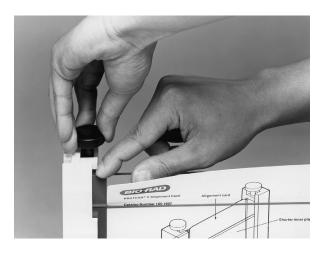
9. Remove the alignment card. Pull the gel sandwich from the alignment slot. **Check that the plates and spacers are flush at the bottom.** If not, realign the gel sandwich as in steps 6-8.
