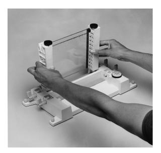
4. With the short glass plate facing the cooling core (and the locating decal on the clamps facing the core), position the gel sandwich so that the grooves in the upper portion of the clamps are fitted onto the locating pins on the central cooling core.\* The gel sandwich should be positioned at an angle of ≤20° with the cooling core. Keeping this angle to a minimum and lubricating the gasket will prevent distortion of the gasket while the sandwich slides into place.
