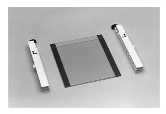
3. Grasp the whole glass plate sandwich firmly with your right hand. With your left hand guide the left clamp onto the sandwich so that the long and short plates fit the appropriate notches in the clamp. Tighten the single screw enough to hold plates in place.
