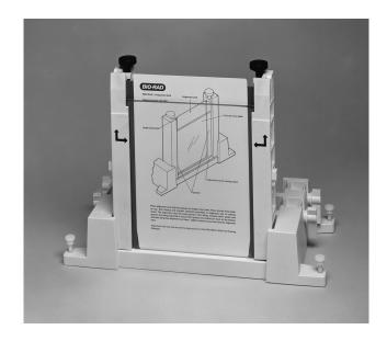
7. Simultaneously push inward on both clamps at the locating arrows, and tighten both clamp screws just enough to hold the sandwich in place. Pushing inward on both clamps at a point below the locating arrows will insure that the spacers and glass plates are flush against the sides of the clamps.
