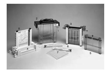
Fig. 1. PROTEAN<sup>®</sup> II xi 2-D cell including tube adaptor. 1. Lower buffer chamber, 2. Lid with electrical leads in place, 3. Cooling core with glass plate sandwich attached and core caps in place, 4. Casting stand with glass plate sandwich in alignment slot, 5. Tube gel adaptor, 6. Sandwich clamps, 7. Buffer dam, 8. Alignment card.
