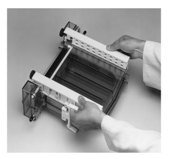
6. Turn the central cooling core to its other side, and repeat steps 1 through 5 to attach the second gel sandwich to it.
