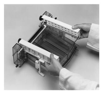
\*Note: The locating pins on the central cooling core must be tightly secured in place to insure optimal pressure during operation. If these pins are vibrated loose during transport or repeated use, the decrease in pressure on the clamp can be enough to allow the cell to leak. If the pins are loose, they can be gently tightened using a coin or screwdriver.
