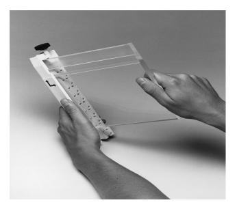
Note: Failure to slide the dam up completely to the top of the clamp will result in an upper buffer leak.
