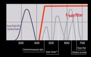
Thanks to the Universal configuration, only one camera filter is sufficient for almost all fluorescent and visible applications.
