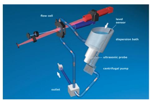
The measurement range of the "X-Flow" module starts at 1 micron. The CAMSIZER XT also analyzes particles larger than 1 mm without difficulty, provided they are kept suspended in the dispersion medium. Depending on the maximum particle size of the sample, measurement cells of up to 4 mm can be used. Agglomerates can be further separated by an integrated ultrasonic probe.
