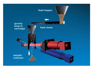
Pourable, not agglomerated samples can be analyzed by using the "X-Fall" plug-in cartridge. In this mode the particles fall from the chute through the field of view of the two cameras accelerated by gravity. Thanks to the comparably low speed of the particles, the large field of view and the high frame rate, the detection efficiency is very high, even for large particles of e. g. 3 mm. Only a few coarser particles in the sample are sufficient for the reliable, reproducible detection.
