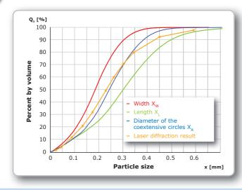
Dynamic image analysis enables simultaneous determination of the size distribution with regards to width  $X_W$  (red), length  $X_L$  (green), and average diameter  $X_A$  (blue). The orange curve shows the result of a laser particle sizer. The laser sizer results correlate well with the average diameter  $X_A$  of the image analysis. However, there are some remarkable differences:
