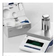
Self-maintenance sets Achieve sustained balance uptime with customized weights and Standard Operating Procedures (SOP).
