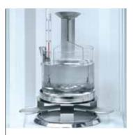
Density Kit Density determination becomes easy with METTLER TOLEDO's density kit for analytical and precision balances.
