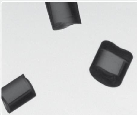
The advantage of the full-frame cameras used by the CAMSIZER P4 for the distortion-free recording of true particle projections is essential when measuring the particle shape.
