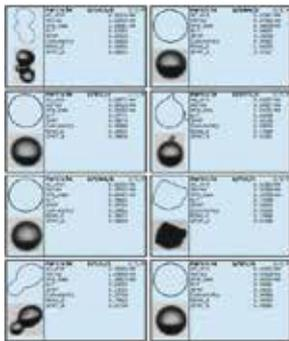
Typical images of glass beads and angular grains with corresponding data
